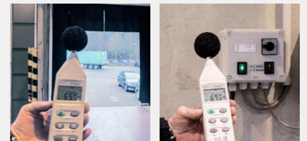
Measurement of the noise level at full load with the air curtain system running
